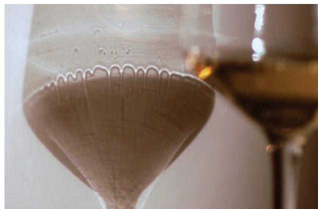
Figure 5. Evidence for the formation of tears (also called legs) on the wall of a glass poured with champagne; tears of champagne are expected to enhance the evaporation of ethanol close to the flute's wall. This photography was done by using the ombroscopy technique. This photograph was taken by Gérard Liger-Belair.
